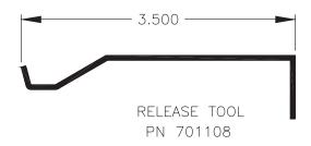
1. Insert tool as shown, near the end of the blade. Push the tool against the blade and rotate.
