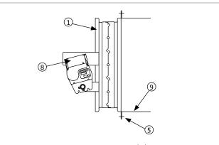
SD35, SD36, SD37, SD50, SD50V(M), SD60, SD60V(M), SD60-2, SD35SS, SD36SS and SD37SS Multiple Blade Smoke Damper Installed within a Flanged Frame or Flanged Sleeve
