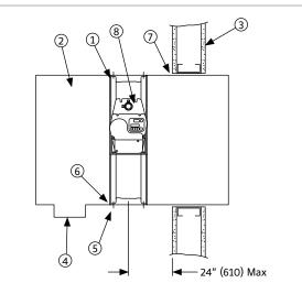
SD35, SD36, SD37, SD50, SD60, SD60-2 SD35SS, SD36SS and SD37SS Multiple Blade Smoke Damper Installed within a Duct or Sleeve
